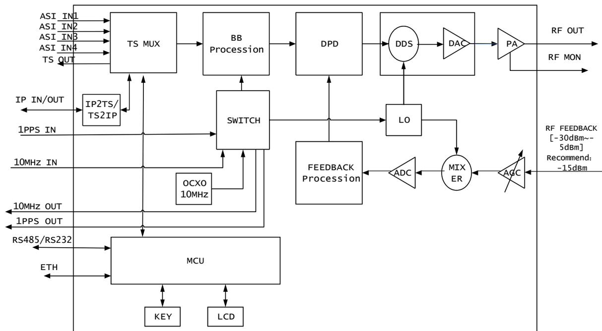
Figure 1.Exciter Diagram
