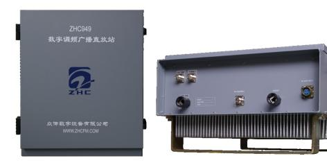
ZHC949-25W digital FM broadcast repeater is a product specially developed for underground parking lots or small tunnels. It has an integrated design for receiving and sending, and the output RF power is 25W. It can forward up to 16 channels of FM broadcast programs at the same time; it can be realized with an emergency broadcast interface. Emergency broadcasting function. Built-in 4G router can realize 4G transmission remote monitoring.
